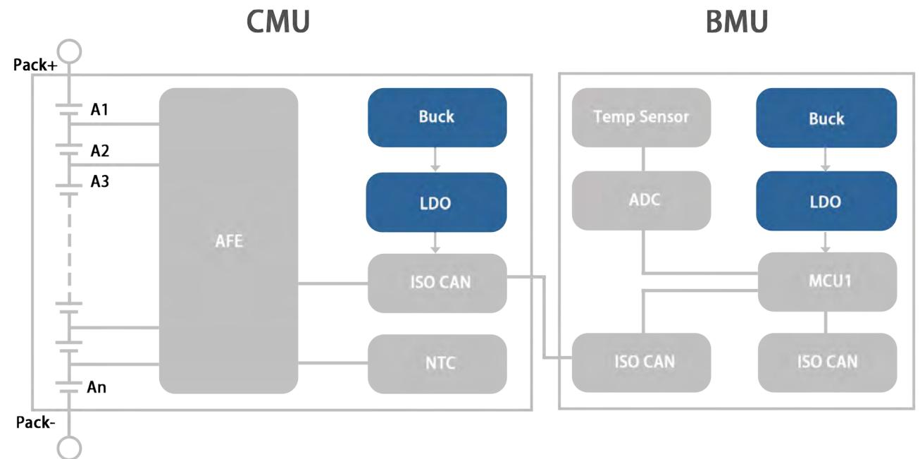
Battery Management System (BMS) enables safe, reliable, and efficient management of battery systems. The system collects battery module data and uploads it to the monitoring platform.
