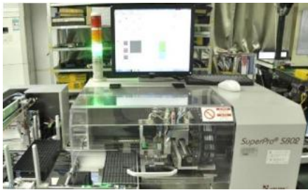
Automatic programming equipment
